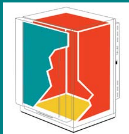
An air jacket with five independent heating elements arranged in three zones surrounds the interior chamber. The microprocessor control system apportions energy to heaters in response to chamber demand and ambient temperature.
