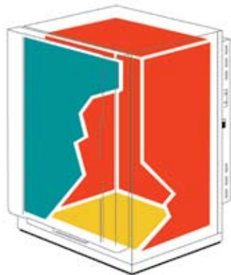
An air jacket with five independent heating elements arranged in three zones surrounds the interior chamber. The microprocessor control system apportions energy to heaters in response to chamber demand and ambient temperature.
